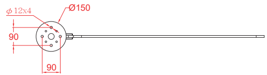
Installation Drawing-Fixing Holes
